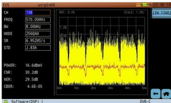
Figure 15: Time-Domain EVS Measurement
