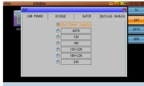
Figure 11: Remote Feeding & Control Signal Setting
