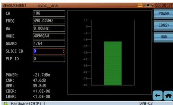
Figure 16: DVB-C2 Signal Quality Measurement
