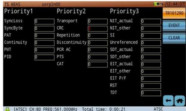
Figure 33: TR101 290 Three-Level Monitoring
