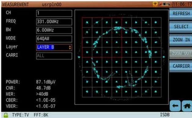
Figure 29: ISDB-Tb Constellation Measurement
