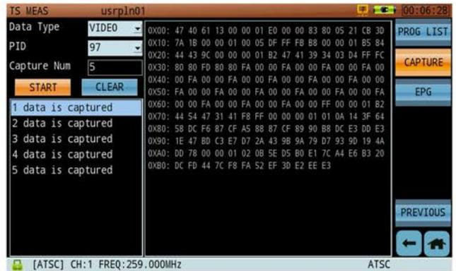
Figure 40: PID Capture
