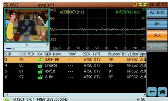
Figure 35: PCR Interval & Accuracy Monitoring
