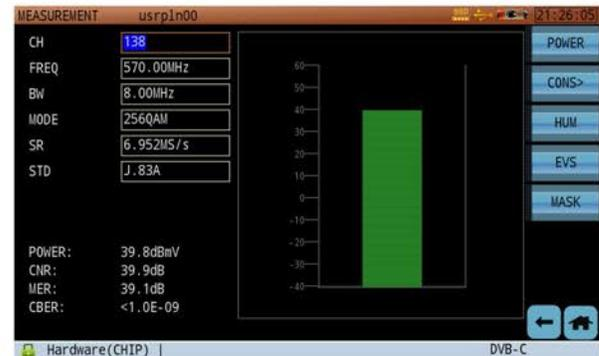
Figure 12: DVB-C Signal Quality Measurement
