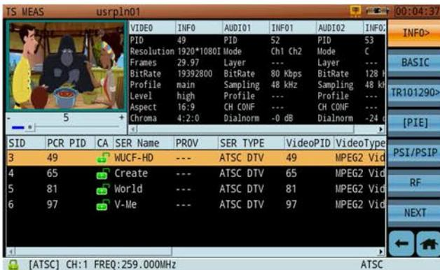
Figure 30: Programs Decode Monitoring & List
