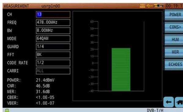
Figure 18: DVB-T Signal Measurement
