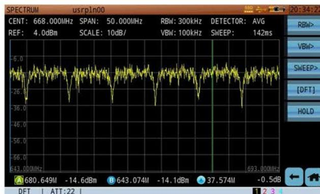
Figure 5: Cable Digital TV Signal Spectrum
